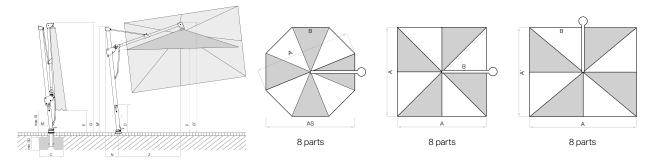
Loose cover max.  $10\,\mathrm{cm}$ , concrete thickness min.  $30\,\mathrm{cm}$  (pay attention to frost depth), Guarantee water drainage
