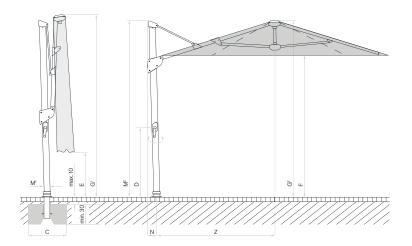
Loose cover max. 10 cm, concrete thickness min. 30 cm (pay attention to frost depth), Guarantee water drainage
