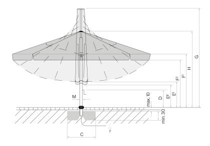
Loose cover max. 10 cm, concrete thickness min. 30 cm (pay attention to frost depth), Guarantee water drainage, Supply line electric.
